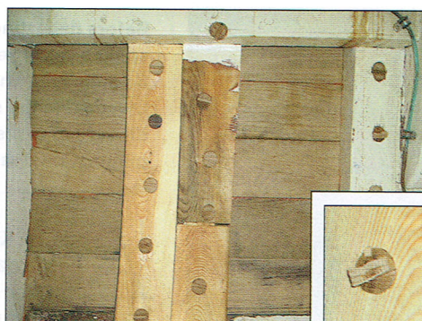
FLEKKERØY has massive scantlings. Her 2"-thick white-oak planking is trunnel-fastened to heavy double-sawn frames, and the trunnels are wedged on the inside (photo right, and inset).
