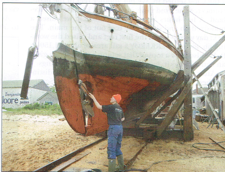
Bjørnar and Klara hauled FLEKKERØY at the Gannon & Benjamin Marine Railway in the spring of 2016 to paint her bottom and topsides. Her 113-hp diesel engine spins a 32" feathering propeller. Dangling here behind the massive outboard rudder is the trim tab of the servo-pendulum self-steering mechanism.
