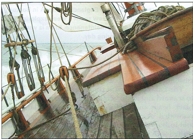
FLEKKERØY charges to windward in a fresh breeze during the 2007 Nordisk Seilas regatta. She carries 1,345 sq ft of sail, which is divided among the mainsail, jib, staysail, and topsail.
